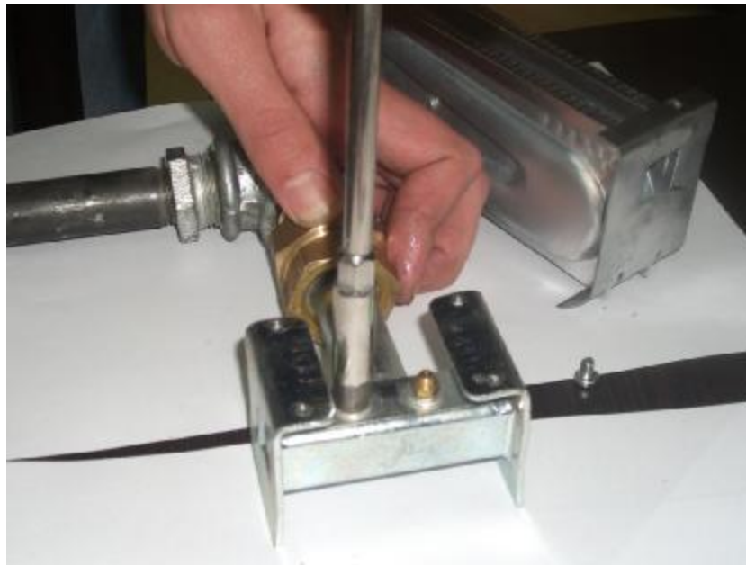
Figure 28 Remove the nozzles with the help of Hex socket number 7.
